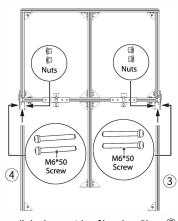
4. Install the lower side of bracket: Place ③ and ④ as shown, fix them with 4 sets of M6 \* 50 screws & nuts.
