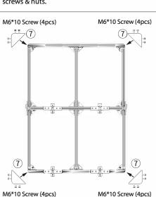
**6.** Install the corner guards of middle bracket: Place ⑦ as shown, fix them with 4 sets of 4 pieces M8 \* 45 screws.
