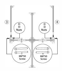
Install the upper side of bracket: Place ③ and ④ as shown, fix them with 4 sets of M6 \* 50 screws and nuts.
