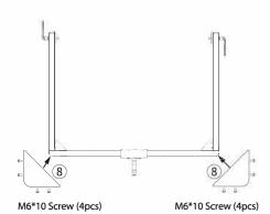
8. Install the corner guards of bottom of bracket: Place (8) as shown, fix them with 2 sets of 4 pieces M8 \* 45 screws.
