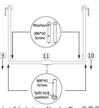
7. Install the bottom of bracket: Place ③ ⑩ ⑪ ⑪ as shown, fix them with 4 sets of M6 \* 50 screws & washers and 2 sets of M8 \* 45 screws & split lock washers.
