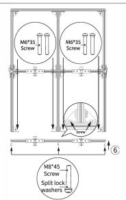
5. Install the lower of bracket: Place ⑥ as shown, fix it with 3 sets of M8 \* 45 screws & split lock washers and 8 sets of M6 \* 35 screws.
