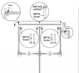
3. Install the upper of bracket: Place ⑤ as shown, fix it with 3 sets of M8 \* 45 screws & split lock washers and 8 sets of M6 \* 35 screws.
