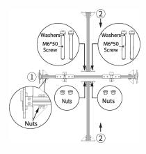
1. Install the middle upper and lower of bracket: Place 1 and 2 as shown, fix them with 4 sets of M6 \* 50 screws & washers and nuts.
